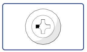
Solution: Check for debris or foreign objects stuck in the engaging section of the Self-Drilling screw.
