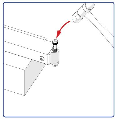
Solution: Place Cap Head Screw into Rail Insert as far as it will go. Place the rail member onto the edge of a solid flat object. While holding the rail firm onto the solid flat object, hit the head of the Cap Head Screw with a hammer until it protrudes through the Rail Insert.
