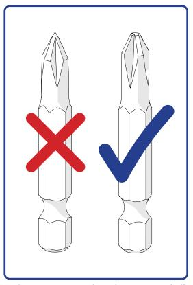
Solution: Ensure that the correct drill bit is being used. The number 2 Phillips Head Bit may need replacing.
