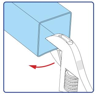
Solution: Hit deformed ends straight with small ball-peen hammer or fold out with adjustable spanner or wrench closed near tight and leaver straight.
