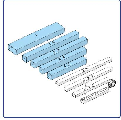
Solution: With a tape measure and marker pen determine each material type and length and write on each member its manual related Item ID & Assembly ID from the material list. This will make the assembly process very easy.
