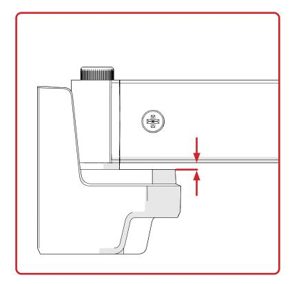
Issue: Cap Head Screw jammed within nut of Universal/Post Connector.
