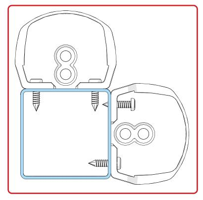
Issue: Screws appear to be clashing internally due to Universal Connectors fitting adjacent and at the same centre measurement.
