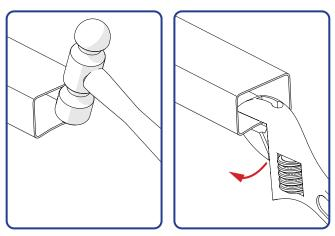
Solution: Hit deformed ends straight with small ball-peen hammer or fold out with adjustable spanner or wrench closed near tight and leaver straight.
