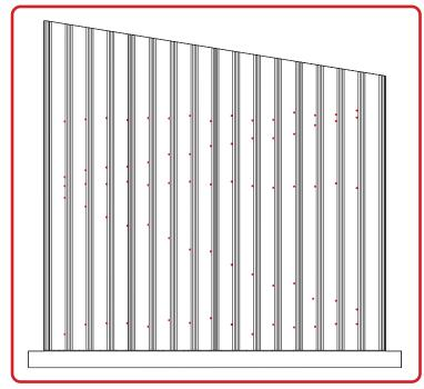
Issue: Cladding screws missing steel framework
