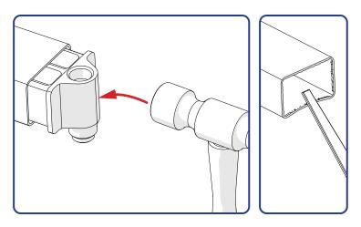
Solution: Light taps on the Rail mid front will help push through internal burr obstructions and mild deformed rail ends. Shaving off Rail Inserts external walls is normal. For 1.6mm thick walled RHS, a file will be needed to remove internal wall burrs.
