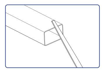
Solution: If desired external burrs can be removed with metal file or mechanical methods such as a sanding disk.
