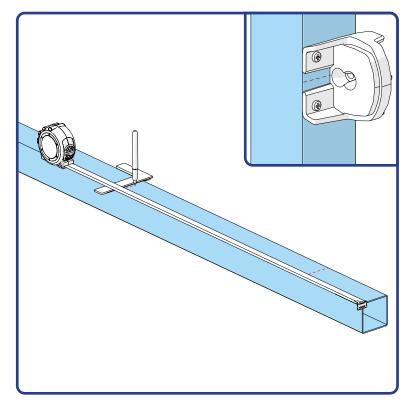
Solution: Use a square to draw straight center lines. Measure twice before fixing Universal connectors or cutting rail members lengths.
