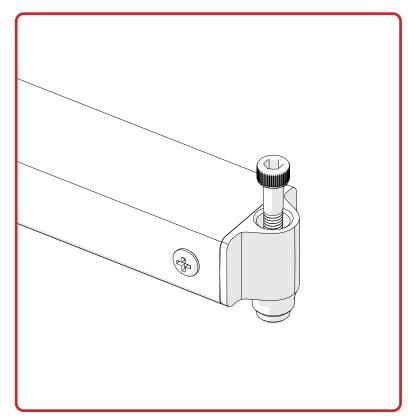
Issue: Cap Head Screw is tight within the hole of the Rail Insert.
