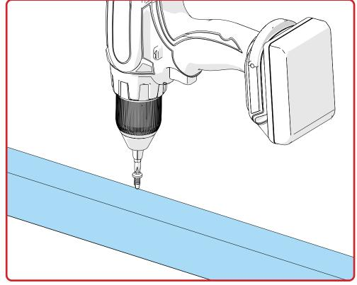
Issue: Drive ends of Self-Drilling screws not engaging properly
