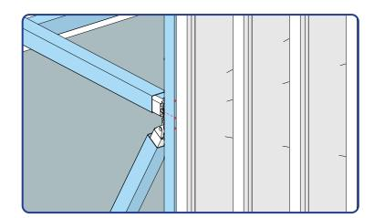
Solution: Hold cladding in place and use a straight edge to transfer centrelines onto the cladding. Mark a line before each rib for screw locations.
