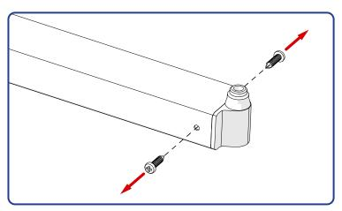
Solution: Remove self-Drilling screws
