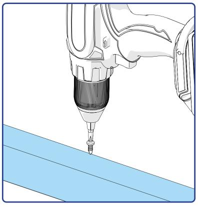
Solution: Apply less downwards force when drilling, drill rotation faster & let the screw do the work.
