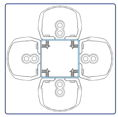
Solution: This is normal as per Kwiktech designs. Ensure self-drilling screws are pushed firmly and true in these situations and the self-drilling screw will naturally deflect past the previously fixed screw it clashes with.
