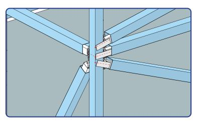
Solution: Mark the centerline of each diagonal & horizontal member on the corner of each vertical post member.
