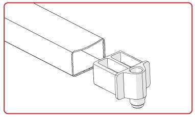
Issue: Deformed and burred 38X25 rail sections due to cutting process and can't insert Rail Inserts properly.
