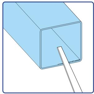
Solution: Remove burrs with a file or with mechanical methods.
