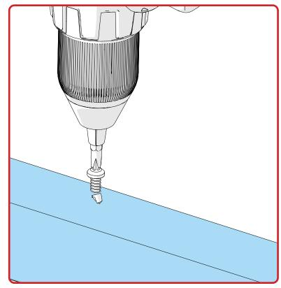
Issue: Self-Drilling screws breaking at their tips when drilling.
