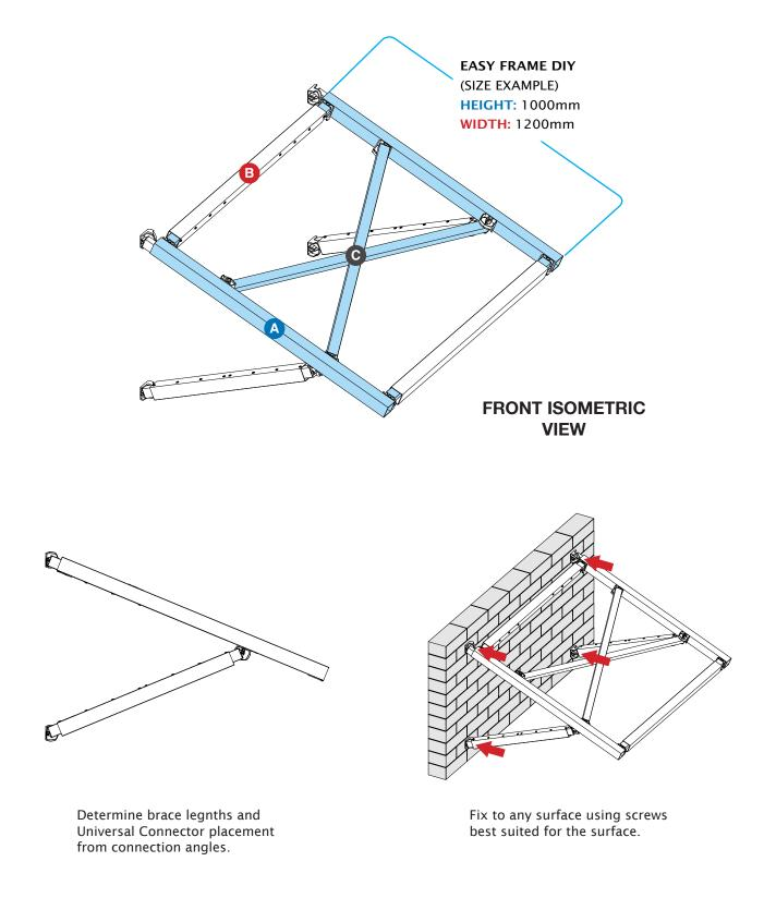
Ensure Brace lengths and Universal Connector placements are the same both sides for a symmetrical build.
