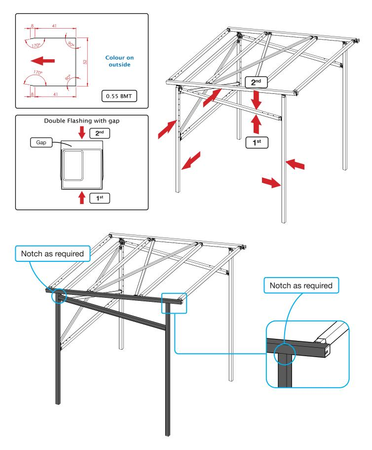
No painting required! Simply select your desired COLORBOND colour, test fit and then glue your flashings on for a flawless finish.
